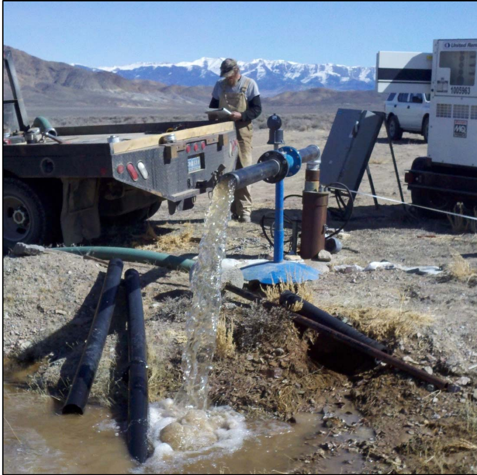
Figure 18.1: Photo of Water Well during Pump Testing
