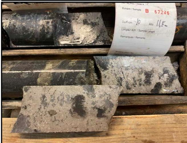
Sample results reported on in this press release were logged and split in the field, bagged, tagged and sealed, then delivered personally by project geologists to ALS Canada Ltd. in Val d'Or, Quebec. The samples were assayed using fire assay for gold with a gravimetric finish.
